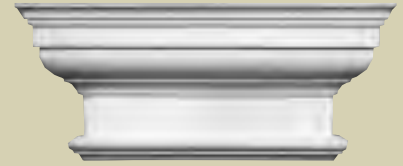
874 TUSCAN PILASTER CAPITAL 18"W x 7 3/4"H x 4 1/2"P TAKES 12 1/2" SHAFT WIDTH
